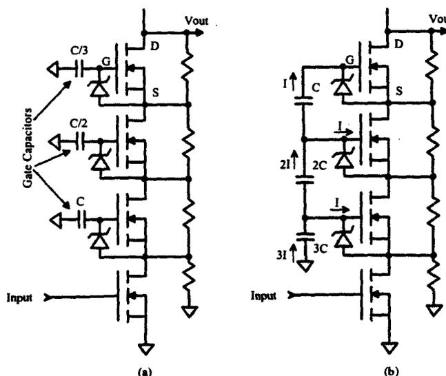
FIG. 1. (a) Basic circuit configuration for stacking power MOSFETs; (b) modified method.
